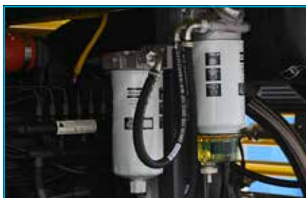
Additional fuel filter as standard to ensure engine protection.
